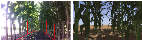
Fig. 10. Real and simulated camera images for corn row following for agricultural robots.
